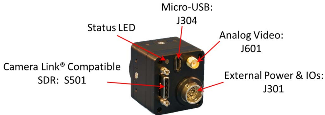
Figure 1 Back Side View of the NOCTURN XL Camera
